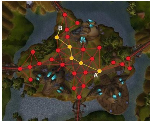
Figure 2.3: Example of a navigation mesh used in a game; the path between A and B is represented as a sequence of yellow links
