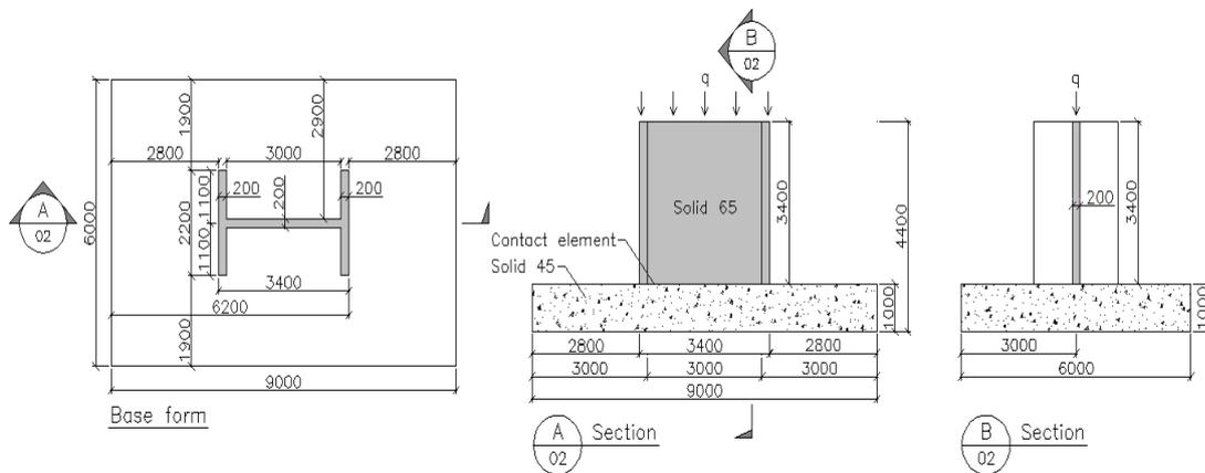
A generic test model represented by a concrete shear wall embedded on gravel cushion foundation. Dimensions are only indicative.
