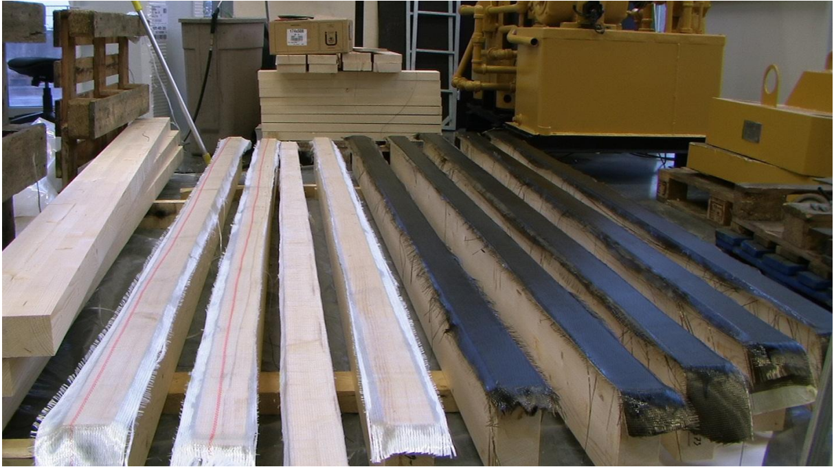
Picture showing glued laminated timber beams strengthened with GFRP (four beams to the left) and with BFRP (five beams to the right)
