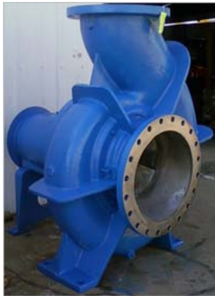
Figure 5. Goulds 316SS Centrifugal Pump 3175 XL (Bid on Equipment, 2009)
